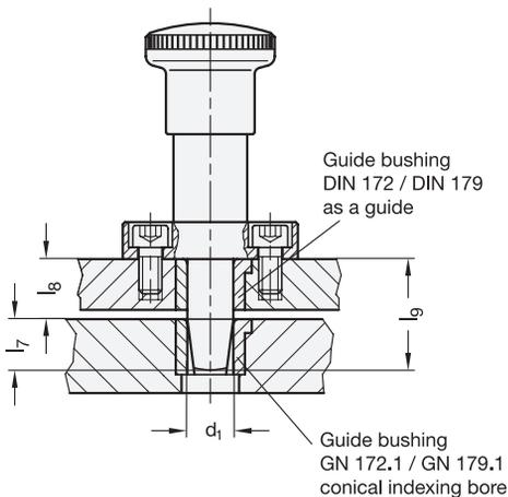
The length  $l_7$  is determined by the penetration depth of the plunger pin into the cone of the bushing.
