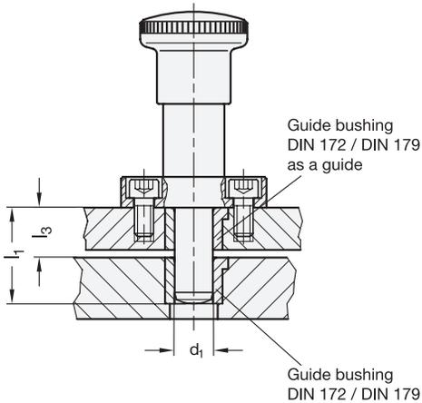
Two different plunger pin lengths  $l_1$  are available for each indexing plunger diameter  $d_1$ .
